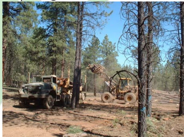
A tractor loads logs onto a hauler during the Fisher restoration treatment this past summer.
